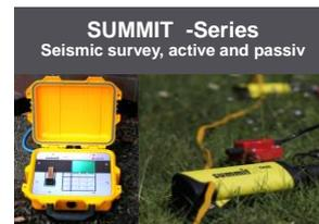
Seismographs are used for monitoring and exploration of structures
