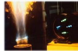
LDA in Turbulent Reactive Flow
